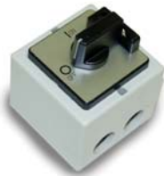
"Elektra" On - Off Switch with box UL/CSA Rated 25 & 35 Amp. Compact 3-1/4" Square x 3-3/4" Deep Enclosure "Versatile Mount".
